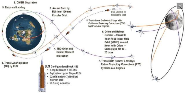
**Figure 5**. Ground sites direct launches and spacecraft flight to and from lunar orbit. (Image courtesy of NASA)
