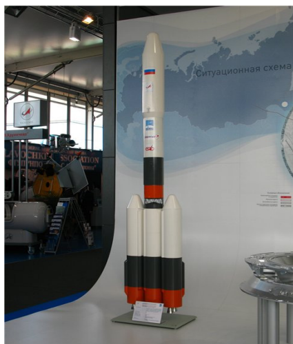
RUS-M Variant-1 approx. 23 metric tons to LEO Variant-3: One non-separable and 4 strap-on boosters
