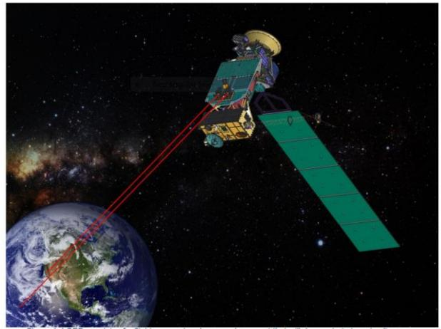
LCRD consists of a flight segment and a ground segment that will demonstrate two simultaneous bidirectional optical links
