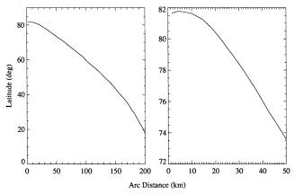
Fig. 4. The latitudinal dependence of the lateral separation between MLS and CloudSat in terms of arc distance between their tracks. Instantaneous, "snapshot", comparisons of smaller mesoscale atmospheric phenomena (10-30 km), as retrieved by both profilers, is apparently possible at high latitudes, in general beyond 78 deg.
