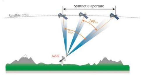
IoSiS satellite imaging geometry with a steerable antenna following the satellite on its orbit path in order to acquire range profiles over a large synthetic aperture path for ISAR processing.
