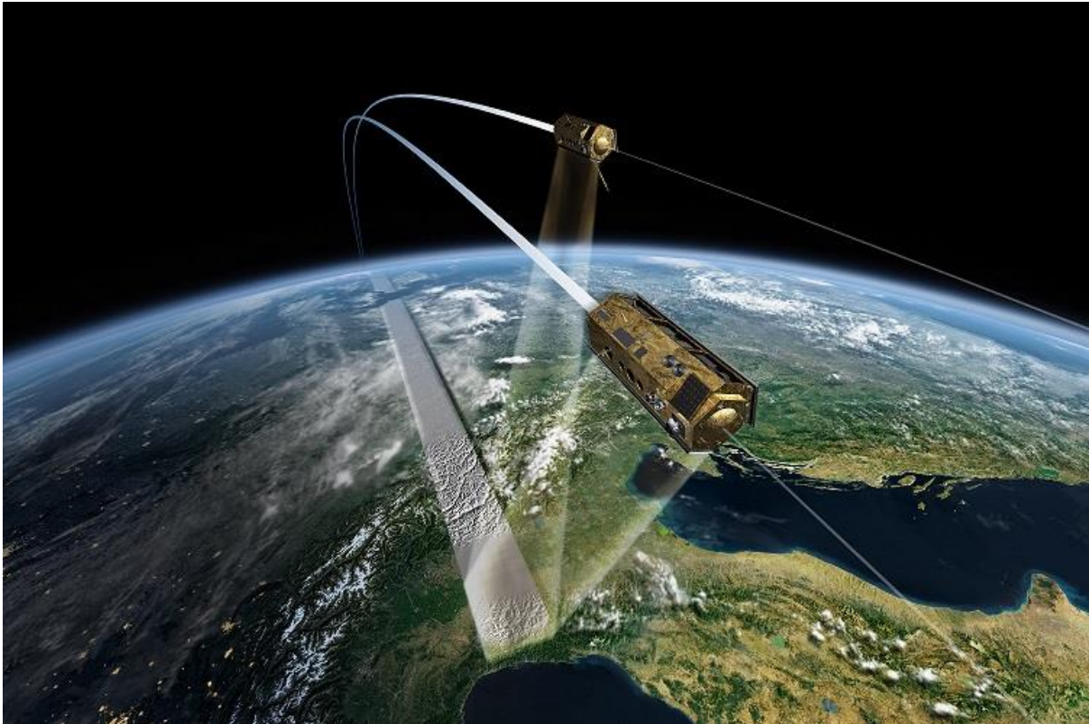
Figure 11: TanDEM-X and TerraSAR-X Spacecrafts in Formation Flying ( Source: DLR )
